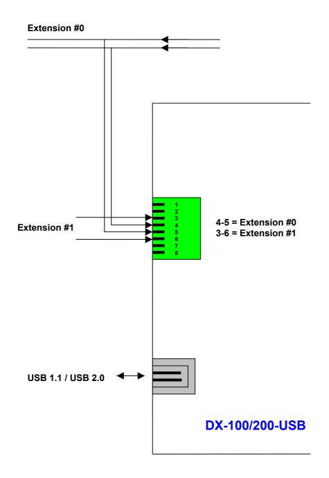
Digital Extension Parallel Mode (RJ-45) for Digital 2-wire PBX Extensions
