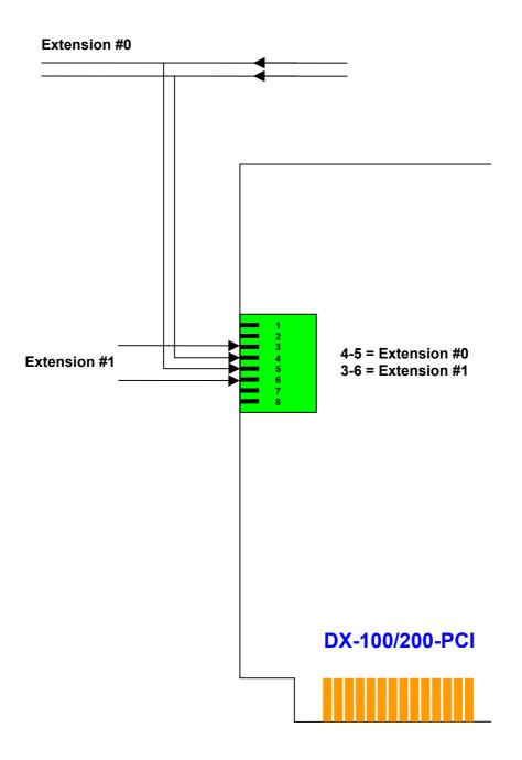
Digital Extension Parallel Mode (RJ-45) for Digital 2-wire PBX Extensions
