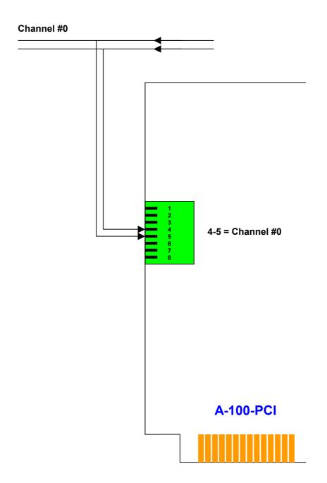
**High-impedance Voltage Detect Parallel Mode (RJ-45)**
